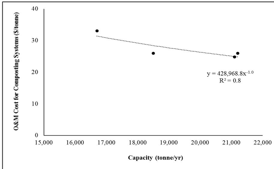
**Figure 7. The O&M cost factor (\$/tonne) as a function of the composting capacity (tonne/yr).**
