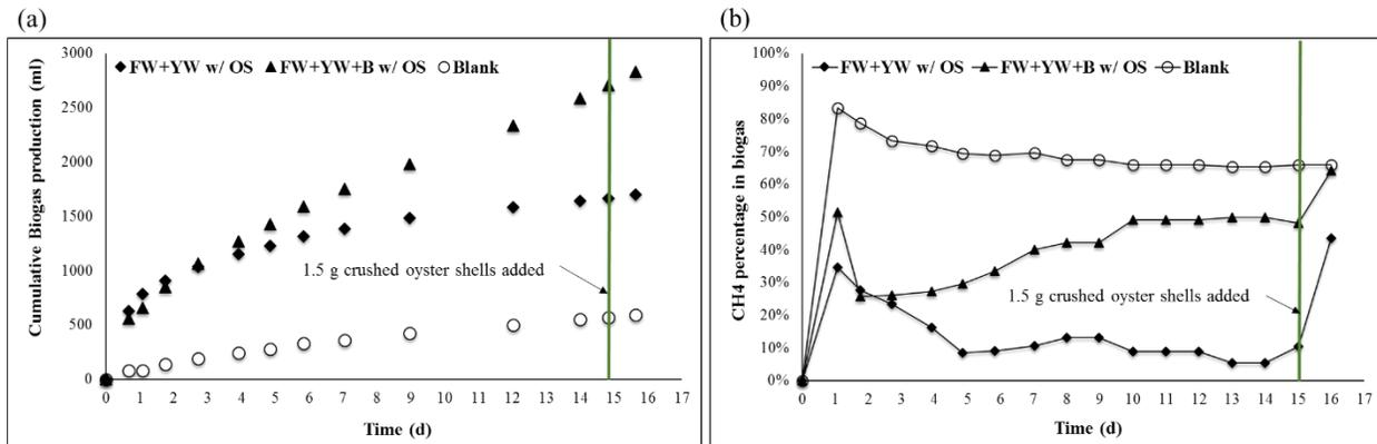
**Figure 2. Biogas production of the HS-AD: (a) cumulative biogas production and (b) CH<sub>4</sub> content in biogas.**
