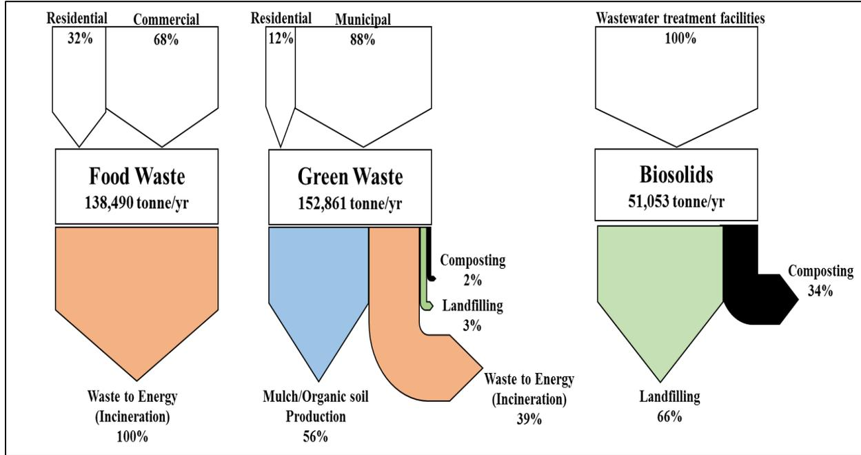
**Figure 6. Production and management flow diagram of FW, GW, and biosolids in 2015.**
